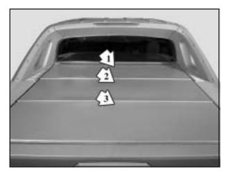
Before removing the cargo panel(s), notice the numbers embossed on the upper center portion of each panel. The panels are labeled 1, 2 and 3. There are also numbered labels on the bottom of the panels. The numbers on the top and bottom of the panels will be used as reference when removing, storing and reinstalling the panels.
